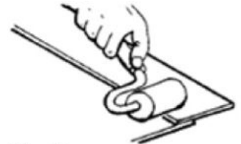
Step D: Roll finished joint
